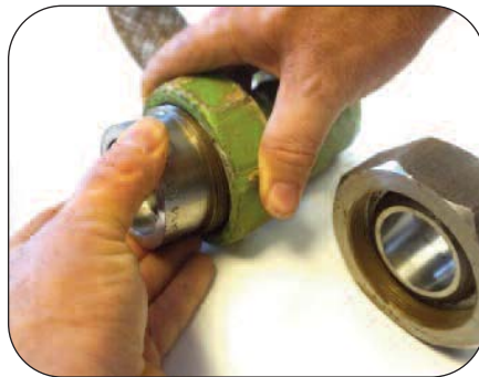
MSS SP 83 2006 3000 lbs thread incompatibility leads to time consuming and costly hose assembly changeouts
